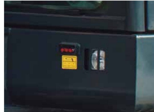
Centralized grease system
