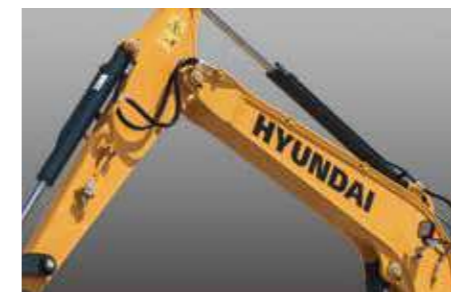
Standard breaker piping
