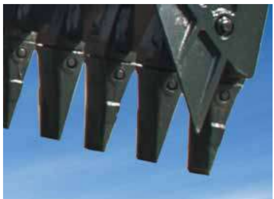
Horizontal type bucket pin
