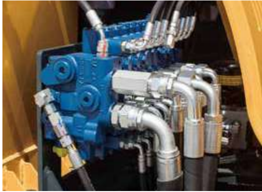
Main control valve on the right side of the cab for noise reduction and heat dissipation.
